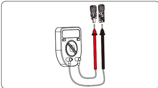
Figure 12-8 Measuring the voltage of PV connectors
