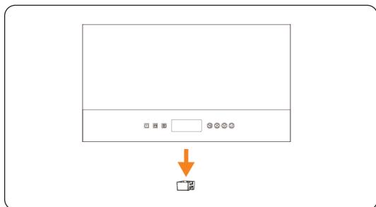
Figure 6-20 Removing the dustproof cover
