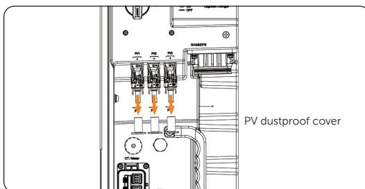
Figure 7-42 Removing the dustproof cover
