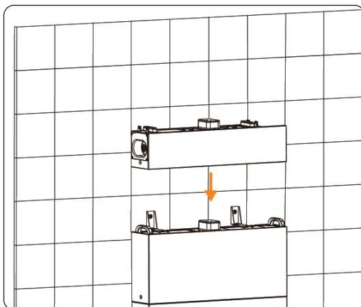
Figure 6-17 Placing the BMS
