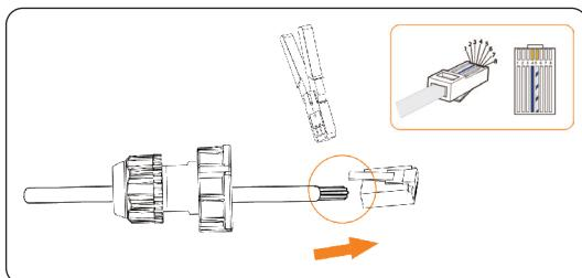
Figure 7-67 Crimping the communication cable for meter
