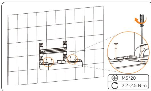
Figure 6-31 Securing the base
