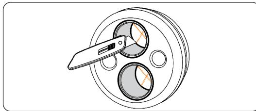
Figure 7-23 Cutting the membrane inside the holes
