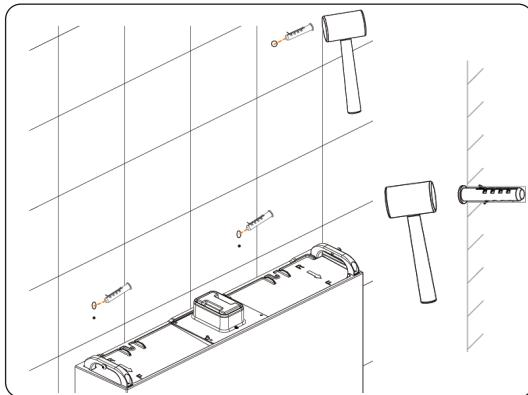
Figure 6-15 Knocking expansion tubes into the wall
