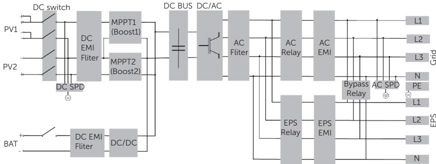
Figure 2-21 4~6 kW system circuit diagram
