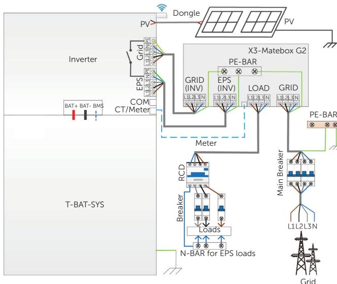
Figure 2-24 System diagram with X3-Matebox G2 for most countries
