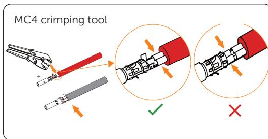
Figure 7-37 Crimping cables with PV pin contacts
