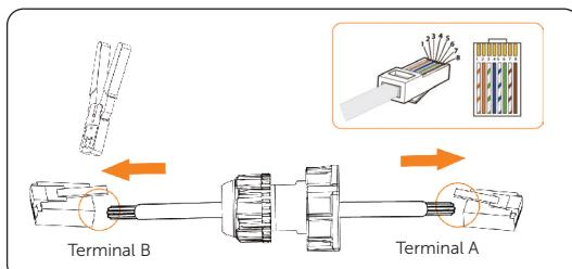
Figure 7-65 Crimping the communication cable for CT
