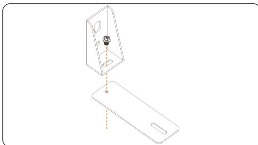
Figure 6-35 Attaching two brackets
