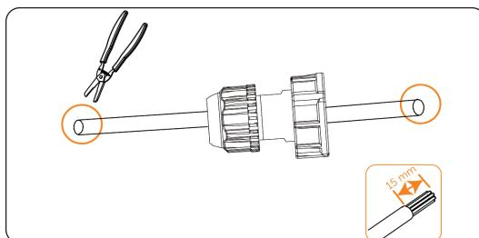
Figure 7-64 Stripping the communication cable for CT
