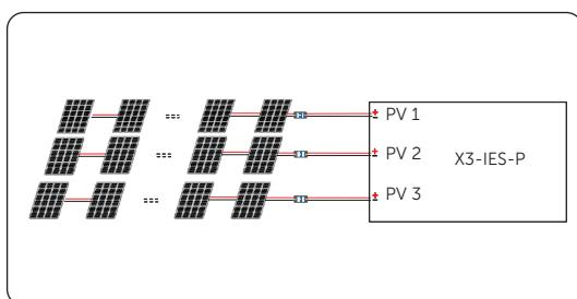
Figure 7-33 "Multi" mode connection diagram
