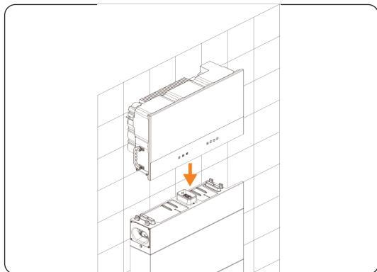
Figure 6-21 Installing the inverter
