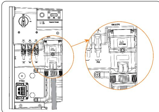
Figure 7-19 Well connected Grid &amp; EPS cables
