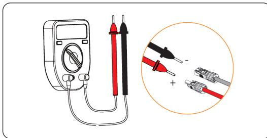
Figure 7-41 Measuring the voltage of PV connectors
