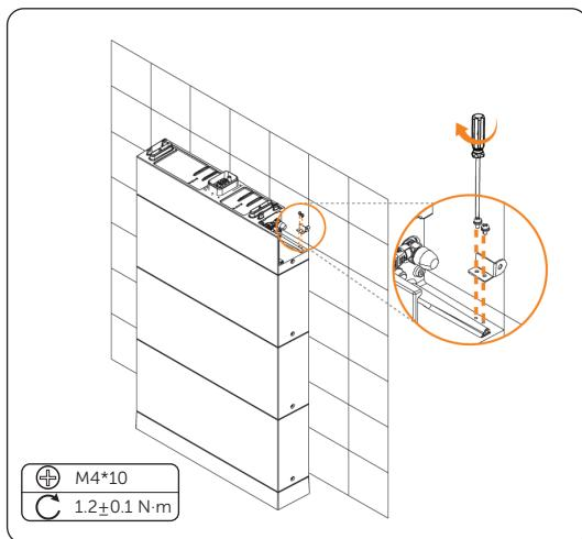
Figure 6-44 Install the anti-tamper bracket
