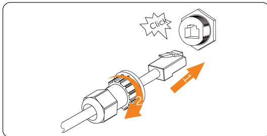
Figure 7-68 Connecting cable to the CT/Meter port
