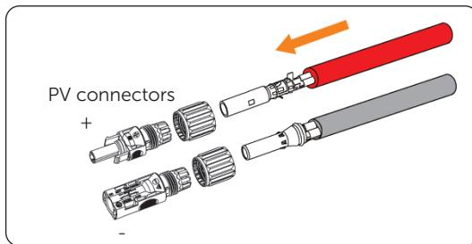
Figure 7-38 Threading PV cables with PV pin contacts connected
