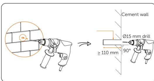
Figure 6-29 Drilling holes
