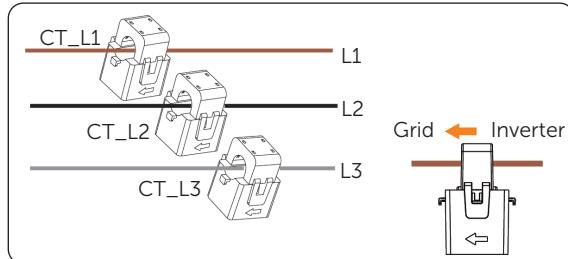
Figure 14-2 Clipping CTs to grid cables
