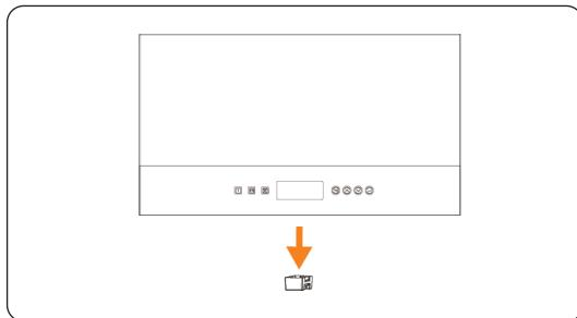
Figure 6-45 Removing the dustproof cover
