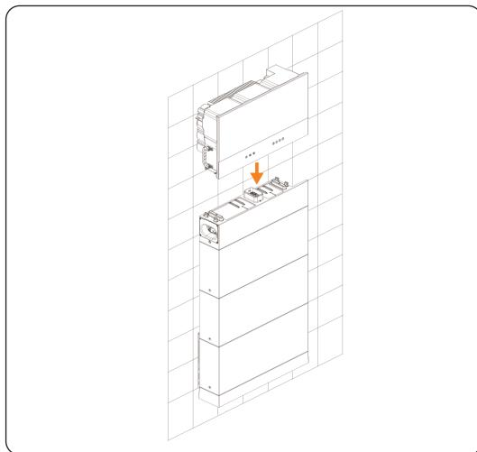
Figure 6-46 Installing the inverter
