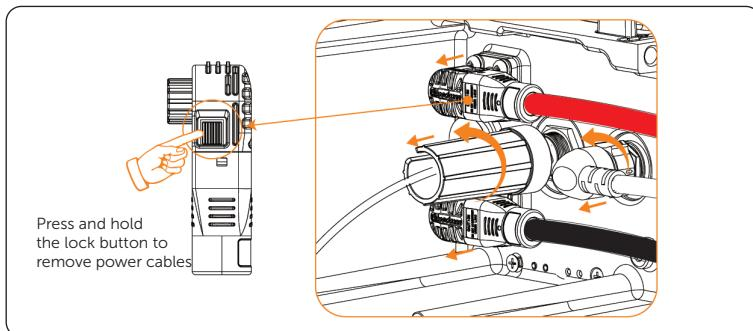
Figure 12-16 Disconnecting battery connectors
