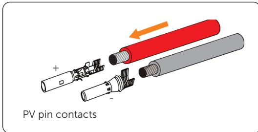
Figure 7-36 Inserting PV pin contacts into PV cables
