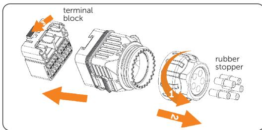
Figure 7-54 Disassembling the communication connector
