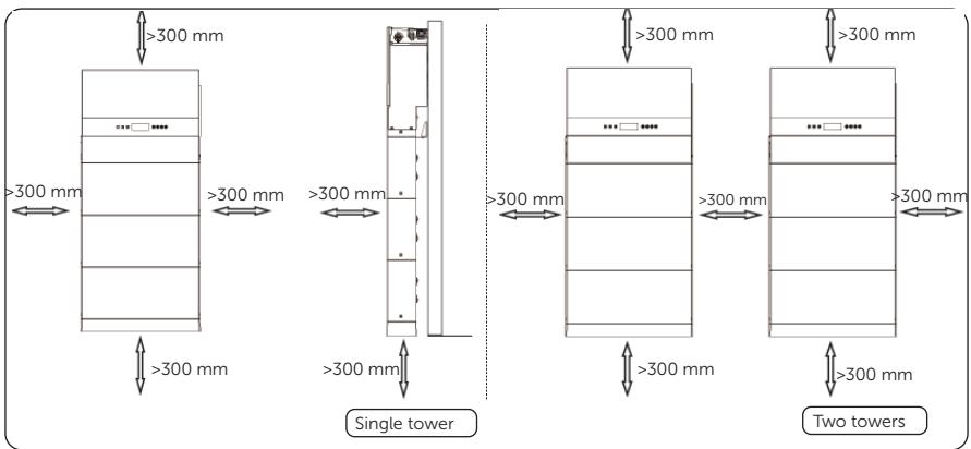
Figure 4-6 Clearance requirement
