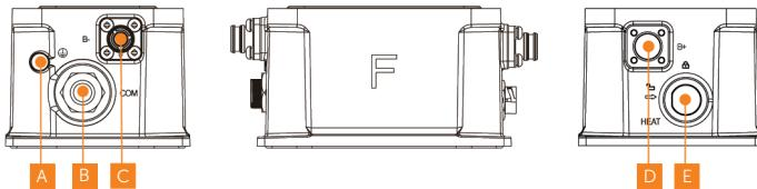
Figure 2-18 Ports of a series box
