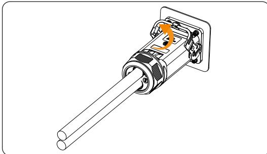
Figure 12-10 Removing the latch of the AC connector
