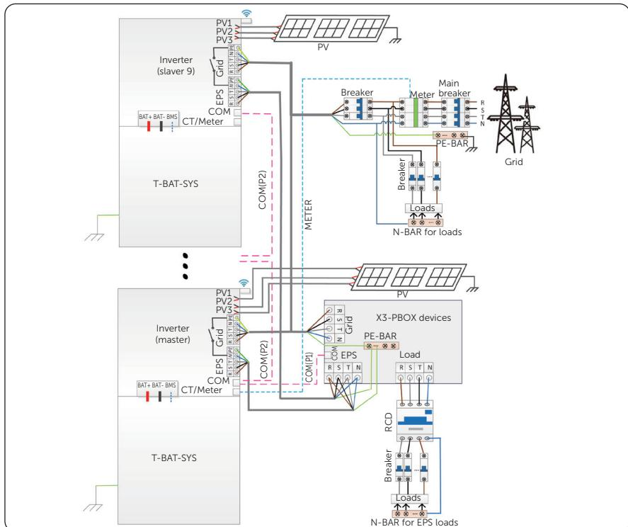
Figure 7-46 System diagram with SolaX X3-PBOX device
