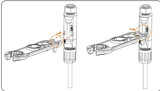
Figure 12-5 Inserting the tool into the PV connector
