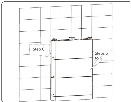
Figure 6-9 Placing battery modules
