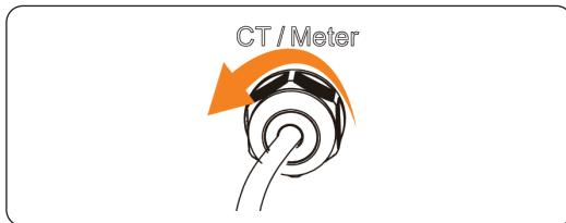
Figure 12-20 Disassembling the meter cable
