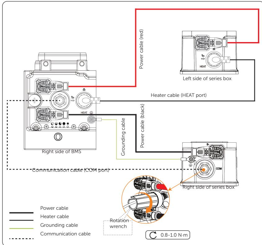
Figure 7-9 Connecting cables
