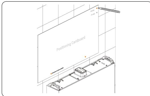
Figure 6-13 Marking the position of the brackets of the inverter
