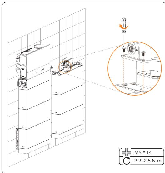
Figure 6-50 Placing the series box
