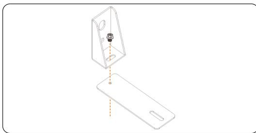
Figure 6-10 Attaching two brackets
