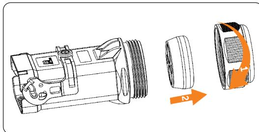
Figure 7-22 Disassembling the AC connector
