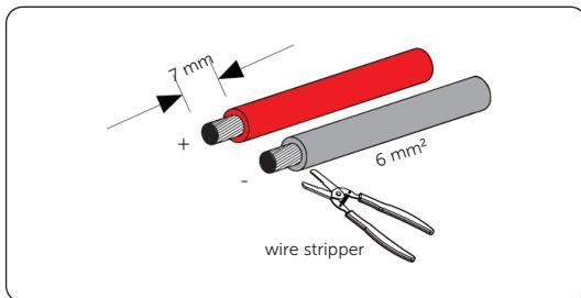
Figure 7-35 Stripping PV cables
