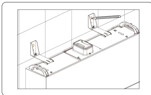
Figure 6-11 Marking the position of BMS
