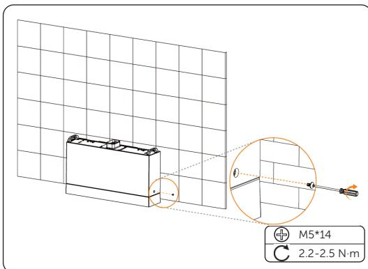
Figure 6-8 Tightening screws
