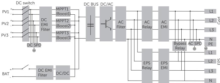
Figure 2-22 8~15 kW system circuit diagram
