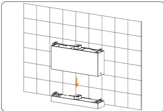
Figure 6-7 Placing the battery module
