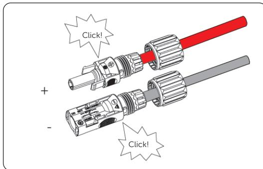
Figure 7-39 Securing PV cables
