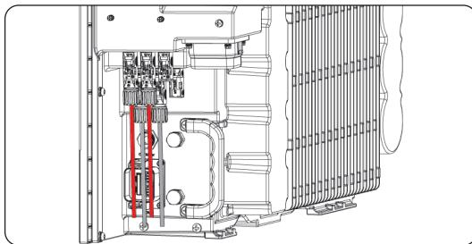
Figure 7-45 Well connected PV cables
