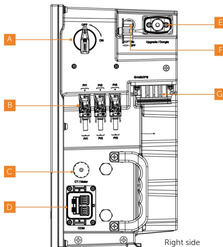
Figure 2-13 Ports of an inverter
