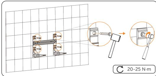
Figure 6-30 Tightening expansion screws
