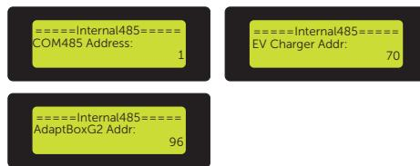
Figure 9-94 Setting the address of the external device
