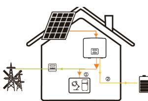
In case of power failure, the system will supply EPS loads through PV and battery. ((The battery must be installed. And the EPS loads must be less than the minimum of the following two values: the sum of the maximum battery discharge power and the maximum PV output power, or the overload limit power of the inverter.)
