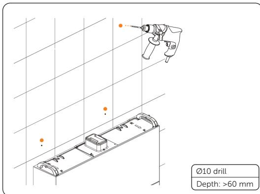
Figure 6-14 Drilling holes
