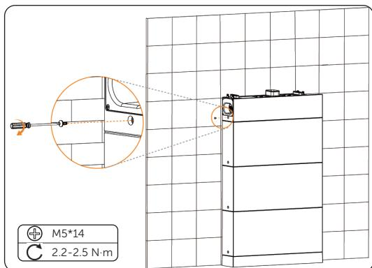
Figure 6-18 Tightening M5 screws
