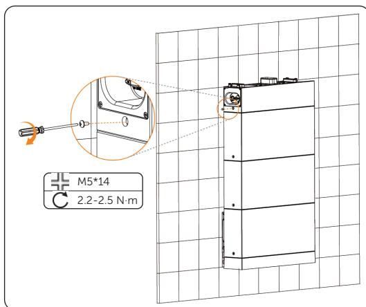
Figure 6-43 Tightening M5 screws
