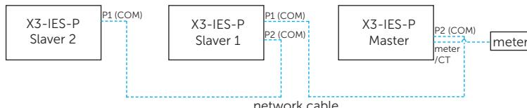
Figure 7-49 Parallel connection without SolaX X3-PBOX device
