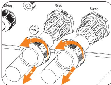
Figure 12-19 Disassembling Grid and Load cables
