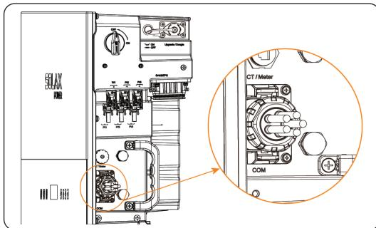
Figure 7-53 Well connected COM port
