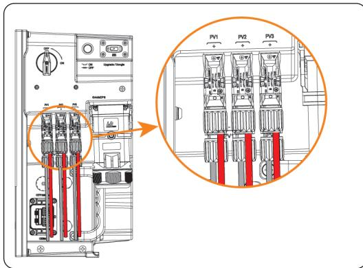
Figure 7-34 Well connected PV cables
