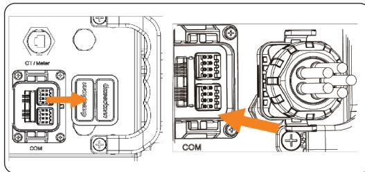
Figure 7-61 Removing the dustproof cover and plugging in the connector
