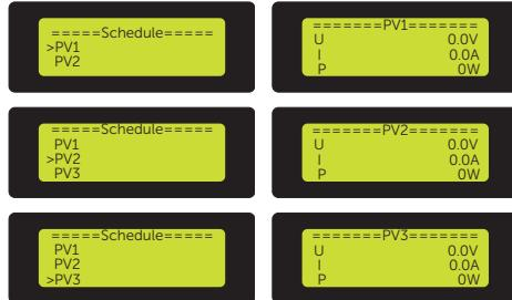
Figure 9-14 Displaying PV1 and PV2 status
