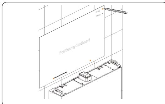
Figure 6-38 Marking the position of the brackets of the inverter
