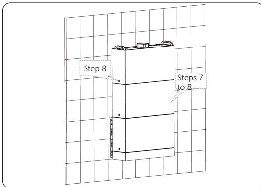
Figure 6-34 Placing battery modules
