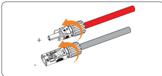
Figure 7-40 Tightening swivel nuts of PV connectors
