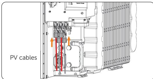
Figure 7-43 Connecting PV cables
