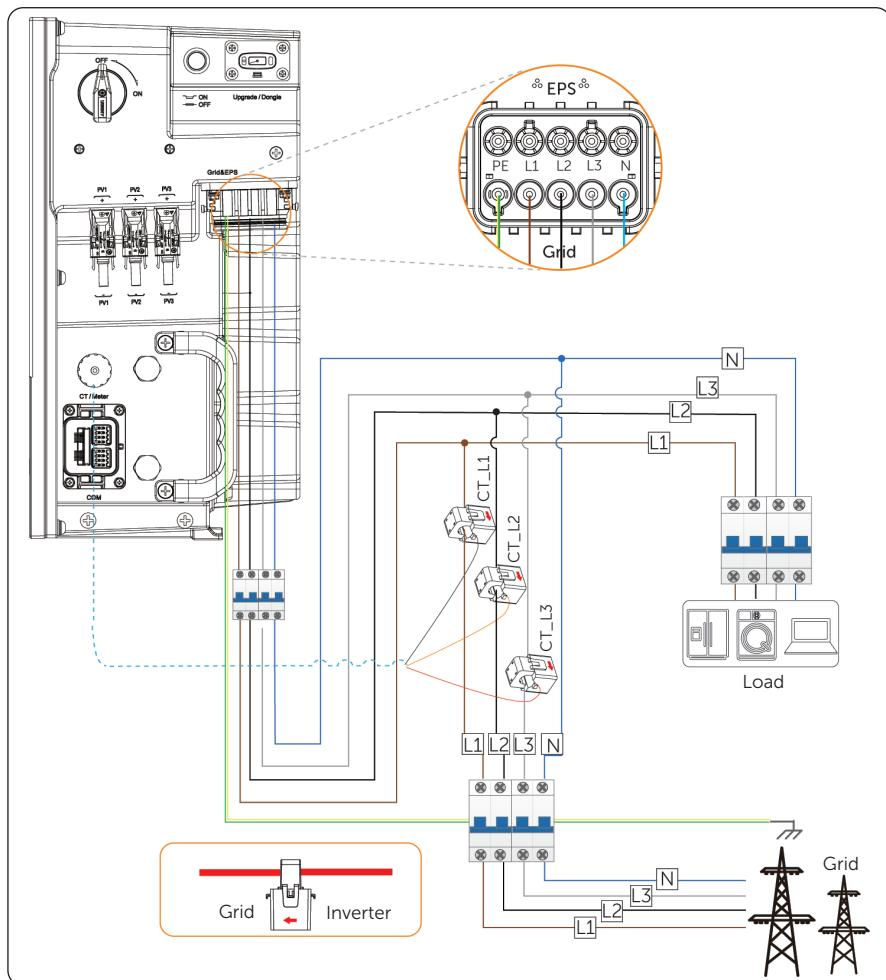
Figure 14-1 System wiring with CT
