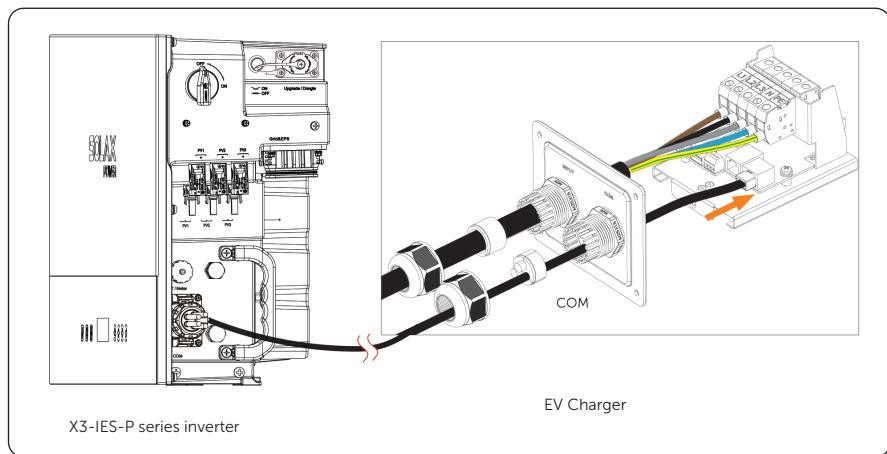
Figure 7-51 Inverter connected with a SolaX EV Charger
