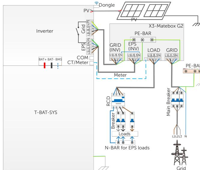
Figure 2-26 System diagram with X3-Matebox G2 for Australia
