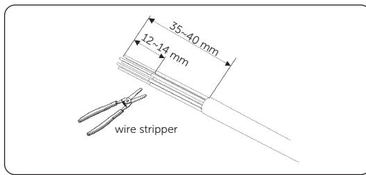
Figure 7-57 Stripping cables
