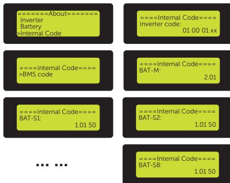
Figure 9-105 Displaying the internal code information
