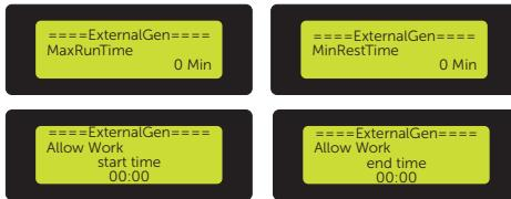
Figure 9-79 Setting MaxRunTime, MinRestTime, allow working period
