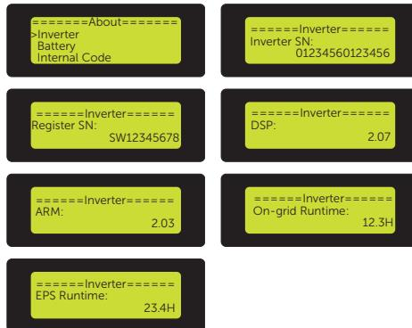
Figure 9-103 Displaying the inverter information
