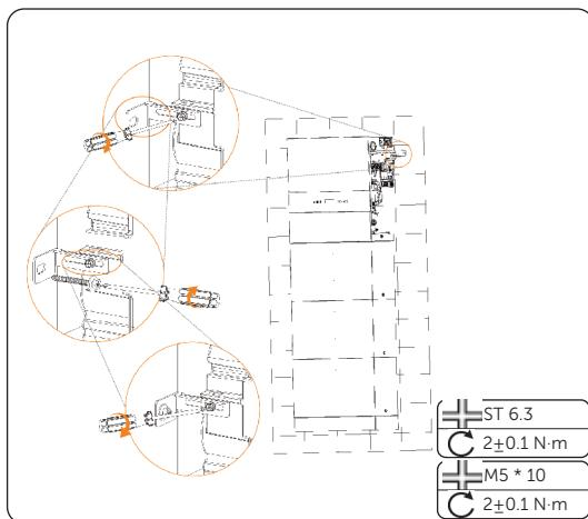
Figure 6-48 Locking the inverter brackets
