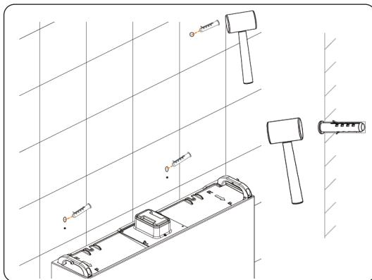
Figure 6-40 Knocking expansion tubes into the wall
