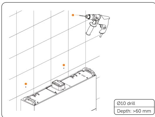
Figure 6-39 Drilling holes
