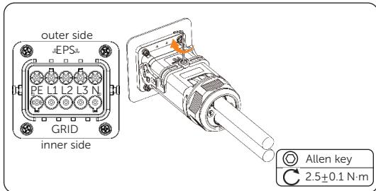
Figure 7-32 Tightening the lock on the AC connector
