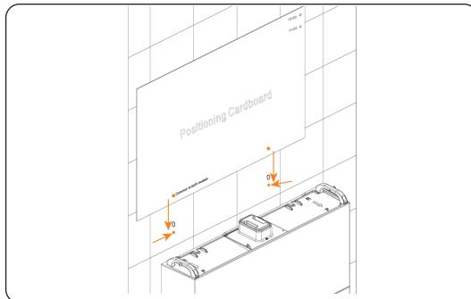
Figure 6-37 Aligning the positioning cardboard with the dots on the wall
