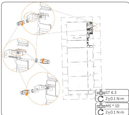
Figure 6-23 Locking the inverter brackets
