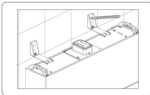
Figure 6-36 Marking the position of BMS
