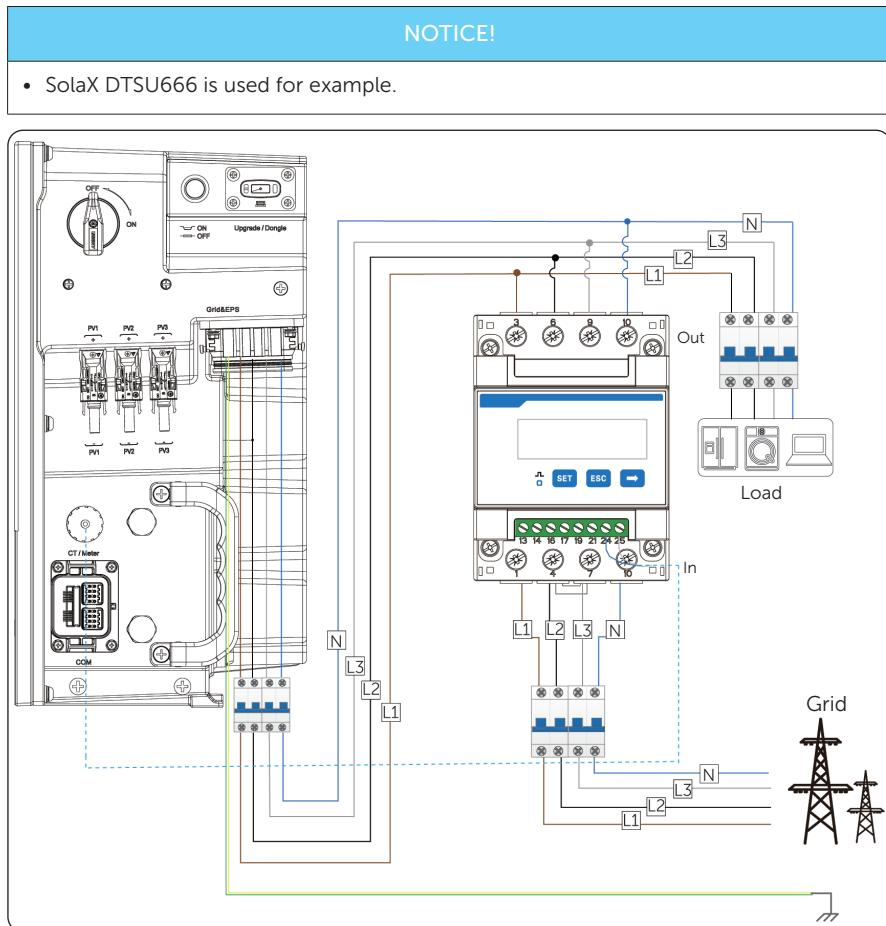
Figure 14-5 System wiring with direct-connected meter
