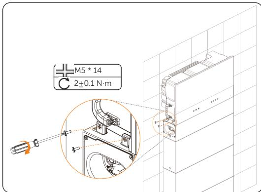
Figure 6-22 Locking the inverter with the BMS
