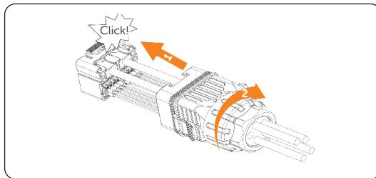
Figure 7-60 Inserting the terminal block into the connector
