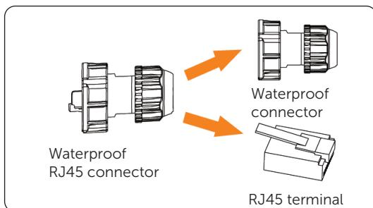
Figure 7-62 Disassembling the waterproof RJ45 connector
