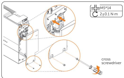
Figure 7-78 Locking the cable shielding board
