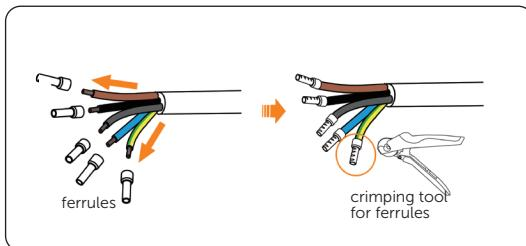
Figure 7-21 Crimping the Grid and EPS cables
