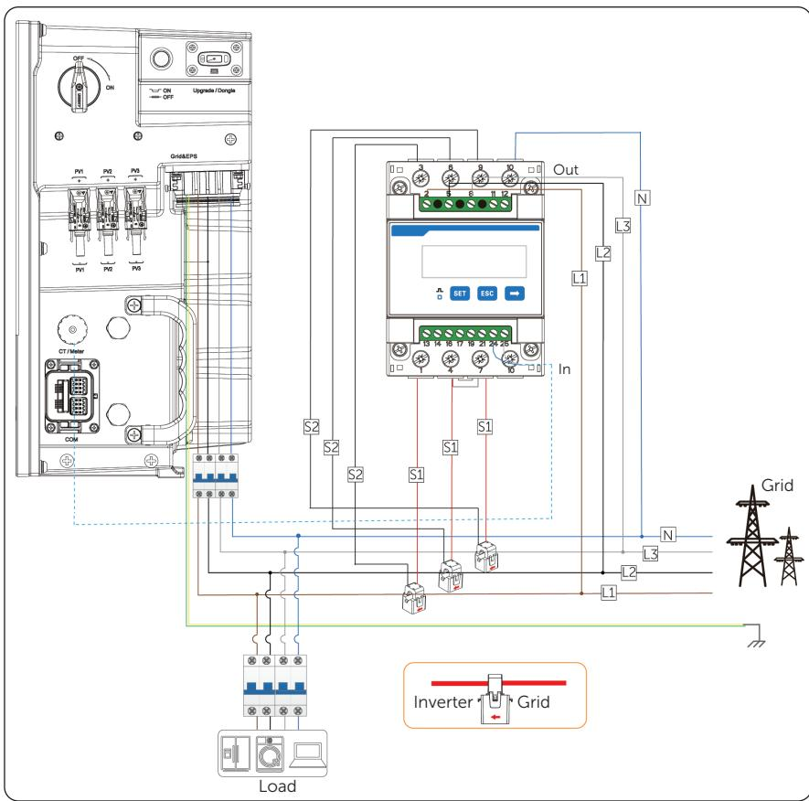
Figure 14-10 System wiring with CT-connected meter
