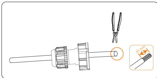
Figure 7-66 Stripping the communication cable for meter
