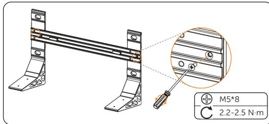
Figure 6-27 Attaching base support and transverse plate
