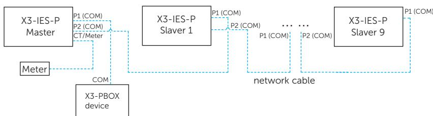
Figure 7-48 Parallel connection with SolaX X3-PBOX device
