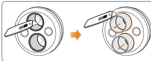
Figure 7-24 Cutting the membrane and tubing inside the holes
