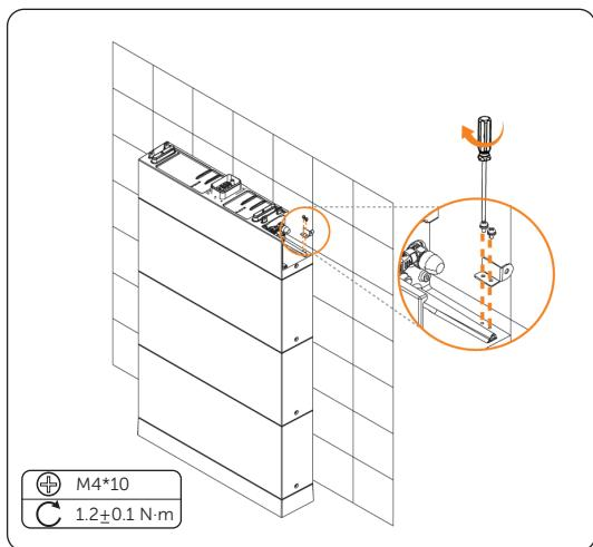
Figure 6-19 Install the anti-tamper bracket
