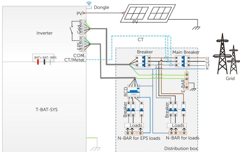
Figure 2-25 System diagram without X3-Matebox G2 for Australia
