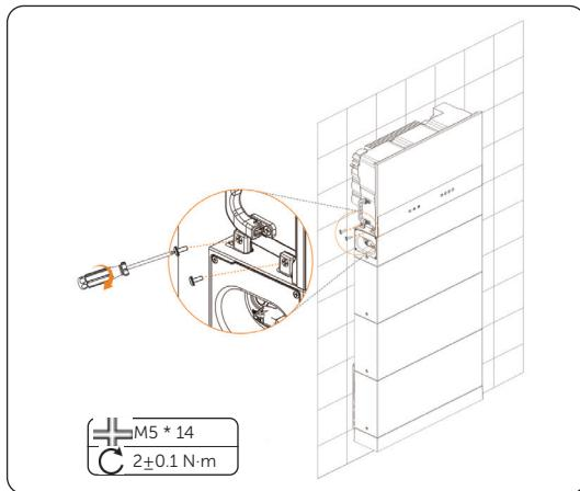
Figure 6-47 Locking the inverter with the BMS
