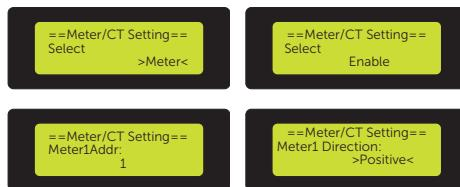
Figure 14-9 Setting meter for the inverter
