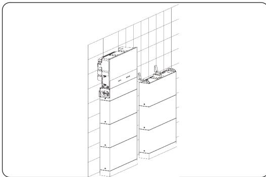
Figure 6-24 Installing two towers
