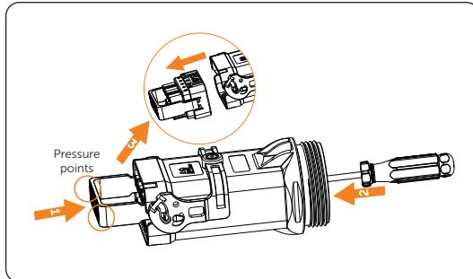
Figure 7-25 Poking the terminal block out of the AC connector
