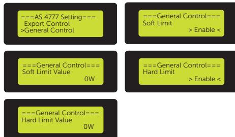
Figure 9-71 Setting general control in AS4777 setting interface
