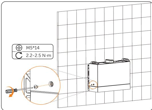
Figure 6-33 Tightening screws
