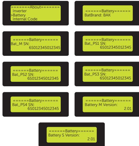
Figure 9-104 Displaying the battery information
