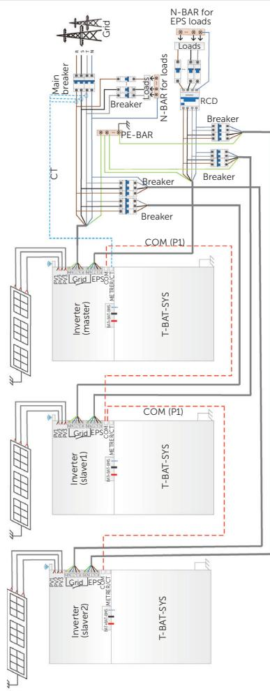
Figure 7-47 System diagram without SolaX X3-PBOX device
