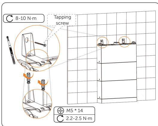
Figure 6-16 Tightening the BMS brackets
