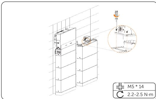
Figure 6-25 Placing the series box
