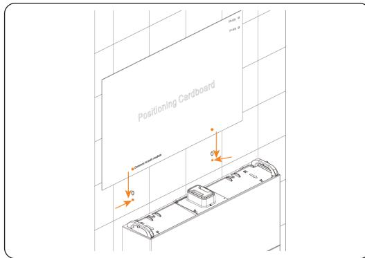
Figure 6-12 Aligning the positioning cardboard with the dots on the wall
