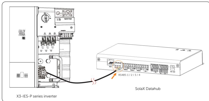
Figure 7-50 Inverter connected with a SolaX datahub
