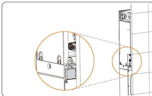
Figure 7-79 Installing the padlock
