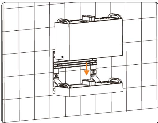
Figure 6-32 Placing battery module
