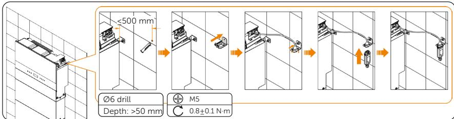
Figure 7-75 Option 2 (for V1 cable shielding board and V1 WiFi connecting cable)
