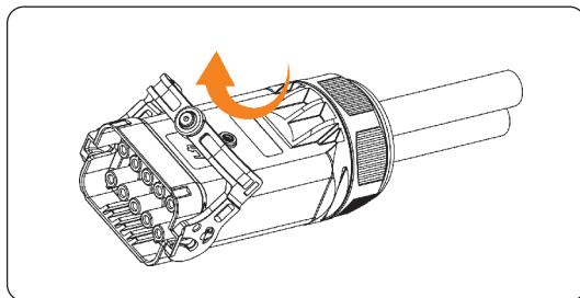
Figure 7-29 Pulling up the latch
