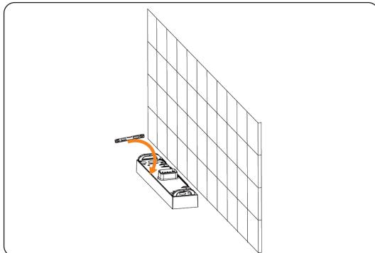
Figure 6-4 Determining whether the base is level
