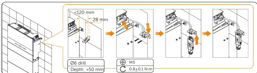
Figure 7-76 Option 2 (for V2 cable shielding board and V2 WiFi connecting cable)
