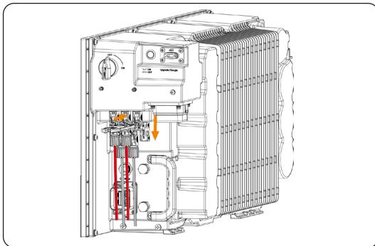
Figure 12-7 Pulling out PV dustproof buckles
