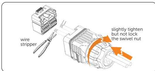
Figure 7-55 Stripping cables
