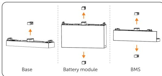
Figure 6-26 Removing dust covers
