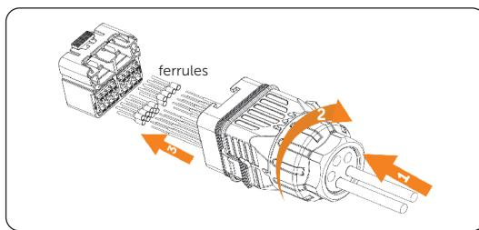
Figure 7-58 Inserting wires into ferrules
