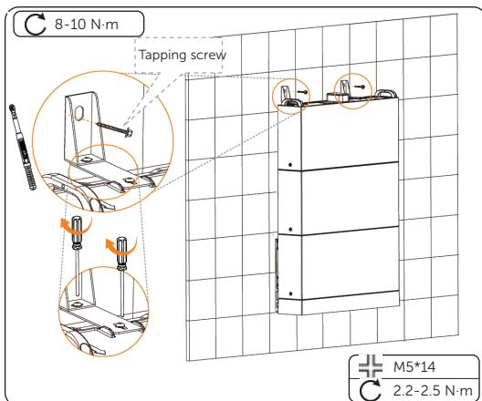
Figure 6-41 Securing the assembled bracket
