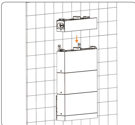
Figure 6-42 Placing the BMS
