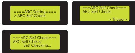
Figure 9-101 Triggering ARC Self Check
