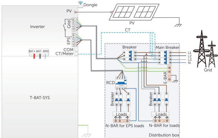
Figure 2-23 System diagram without X3-Matebox G2 for most countries
