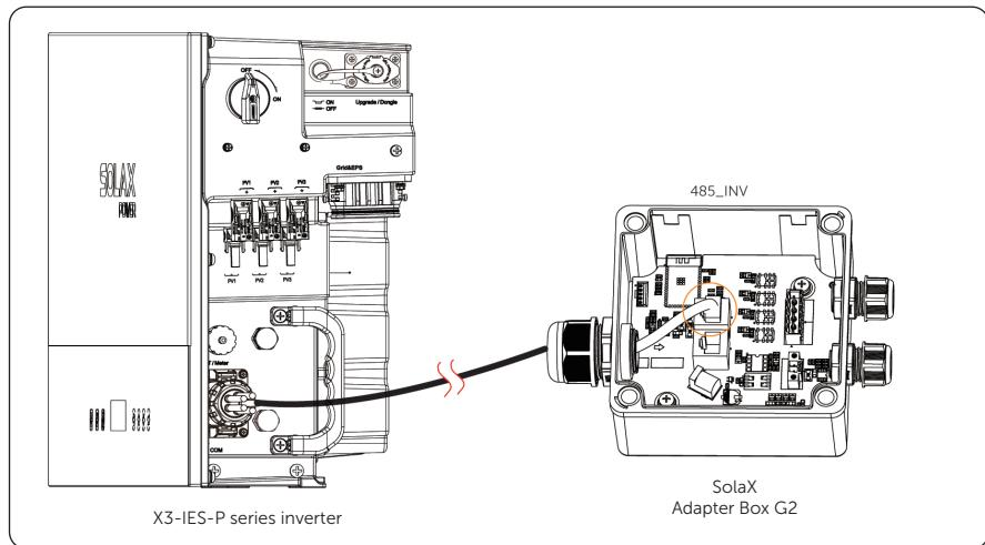
Figure 7-52 Inverter connected with a SolaX Adapter Box G2
