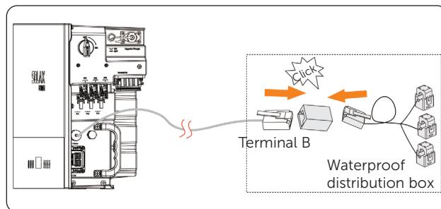
Figure 14-3 Connecting the inverter to the CT
