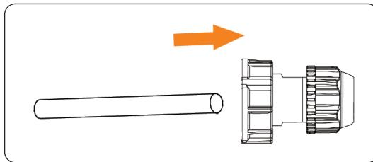
Figure 7-63 Threading the communication cable
